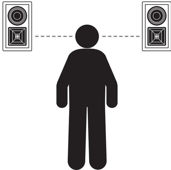
*If the speakers need to be placed high, mount them so that the horn tweeters are on the bottom and are at ear level when the listener is standing up.*
