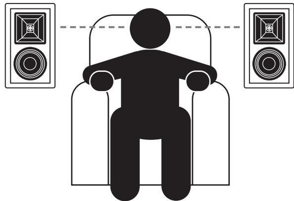
*For best imaging, mount speakers so that the horn tweeters are on the top and are at ear level when the listener is seated.*
